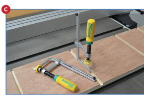
3. The head of the MATCHFIT Dovetail Clamp is forged 1/2" wide with 14° angles on each side so it slides easily within a 1/2"x14°x3/8" deep dovetail slot that you cut wherever needed.
