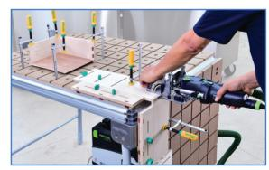
Build a gridded dovetail work table with horizontal and vertical work surfaces to make accurate, repeatable 90° joinery and build drawers in less than half the time.
