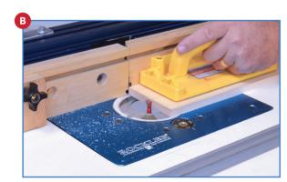
2. Create a dovetail groove in your workpiece using a router with the 1/2" diameter, 14° dovetail router bit. B
