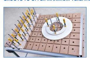
Build a dovetail groove grid work surface. For gluing and assembly projects, apply even clamping pressure on all four sides while the workpieces are clamped completely flat on the work table, including from the center on circular projects.
