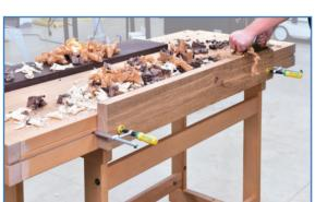
Groove dovetails into your workbench to create the ultimate end vice for large workpieces.
