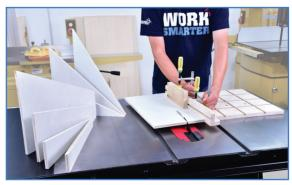
Build a 360° dovetail table saw sled. The fence can be locked from 0° to 360° in any groove. Cut panels at any angle or width that fit on the sled. A ZEROPLAY Miter Bar or equivalent should be installed on the 360° dovetail sled.
